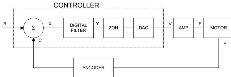
Figure 10.4: Functional Elements of a Motion Control System
