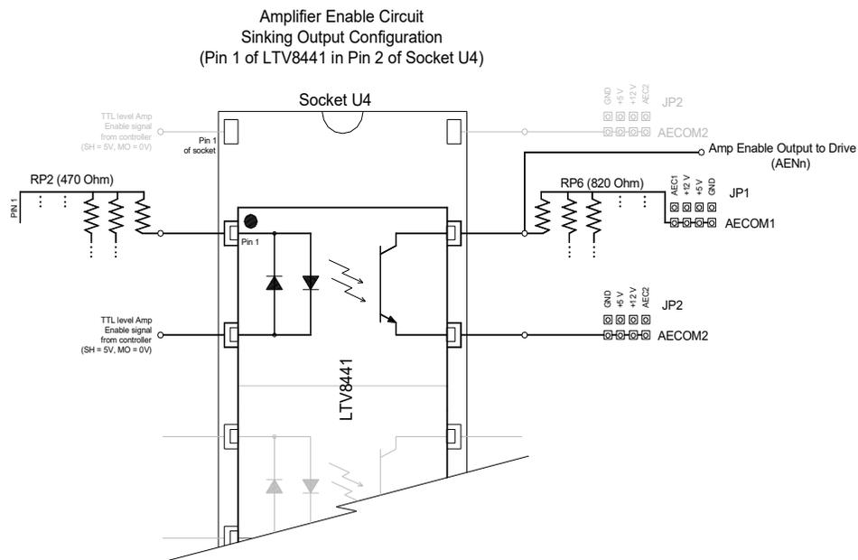
Figure 3.8: Amplifier Enable Circuit Sinking Output Configuration
