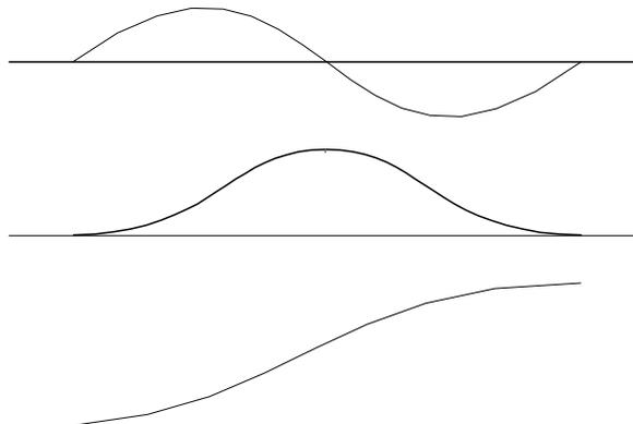
Figure 6.19: Velocity Profile with Sinusoidal Acceleration
