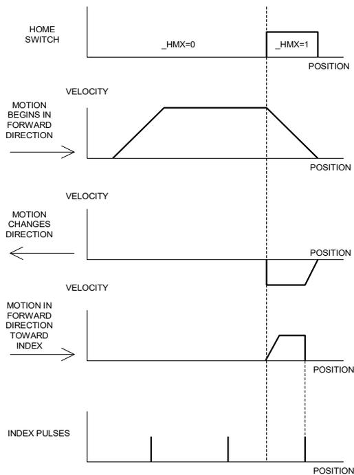
Figure 6.21: Homing Sequence for Normally Closed Switch and CN,-1
