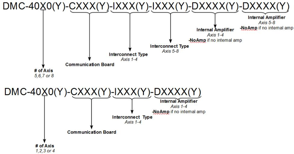
Figure 1.3: Layout of a complete DMC-40x0 part number
