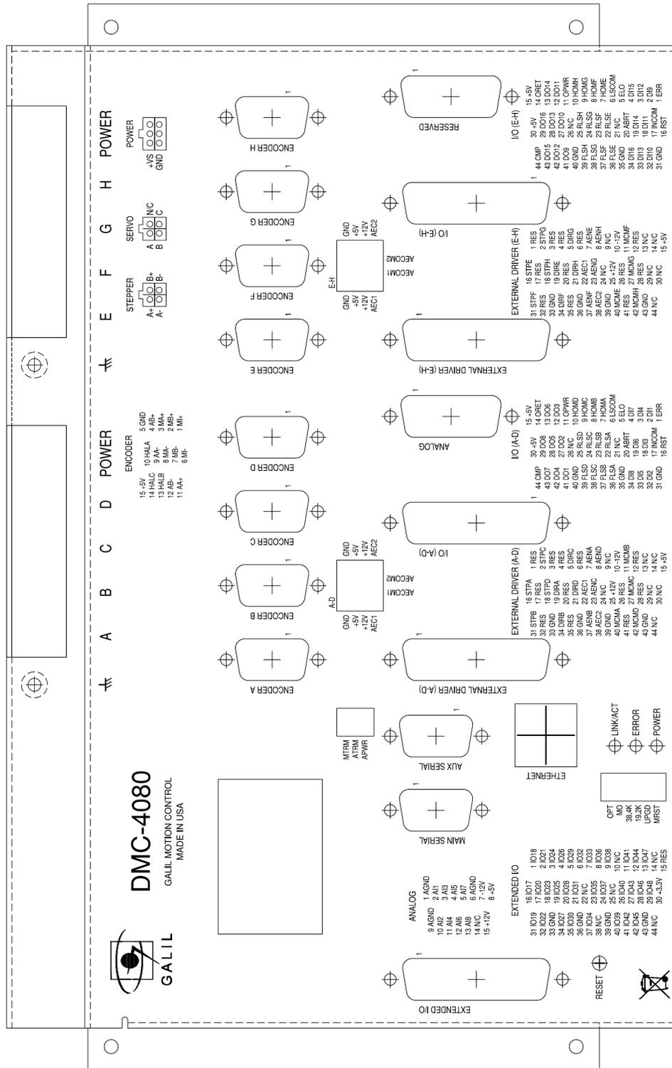
Figure 2.2: Outline of the of the DMC-40x0, 5-8 axes model
