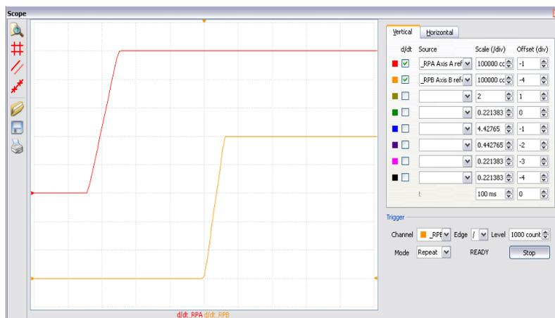
Figure 6.12: Velocity (counts/sec) vs. Time (msec) Ramped Gearing
