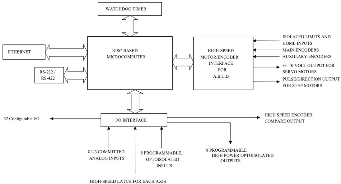
Figure 1.4: DMC-40x0 Functional Elements
