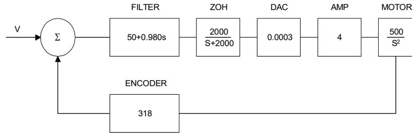
Figure 10.7: Mathematical model of the control system
