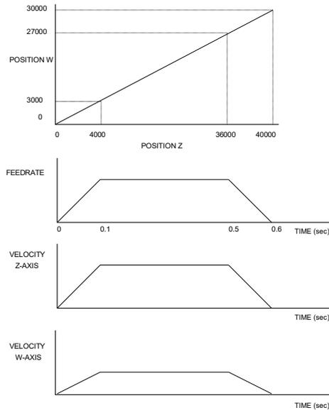
Figure 6.6: Linear Interpolation
