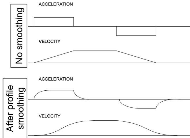
Figure 6.20: Trapezoidal velocity and smooth velocity profiles
