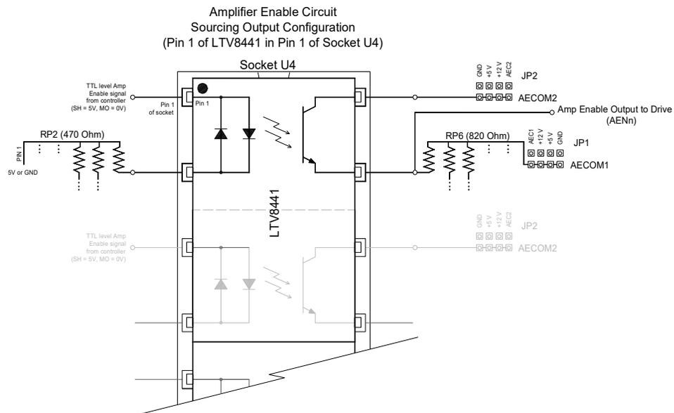
Figure 3.9: Amplifier Enable Circuit Sourcing Output Configuration
