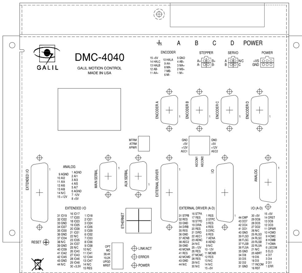
Figure 2.1: Outline of the the DMC-40x0 1-4 axes model
