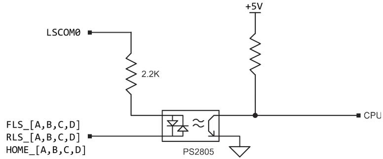
Figure 3.3: Limit Switch Inputs for Axes A-D
