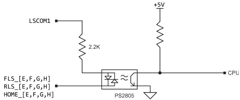
Figure 3.4: Limit Switch Inputs for Axes E-H
