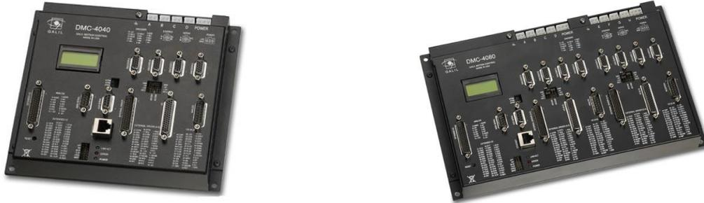
*Default 1-4 axes model (left), default 5-8 axes model (right)*
