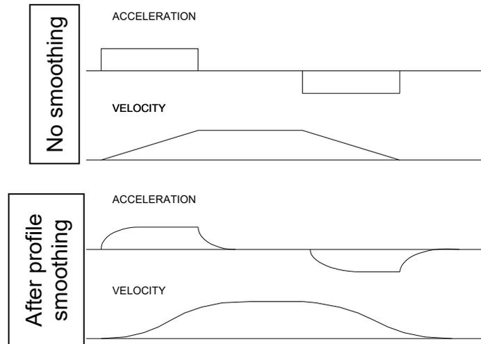
Figure 6.21: Trapezoidal velocity and smooth velocity profiles
