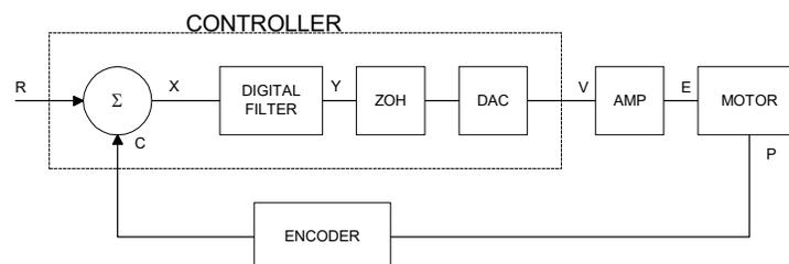
Figure 10.3: Functional Elements of a Motion Control System
