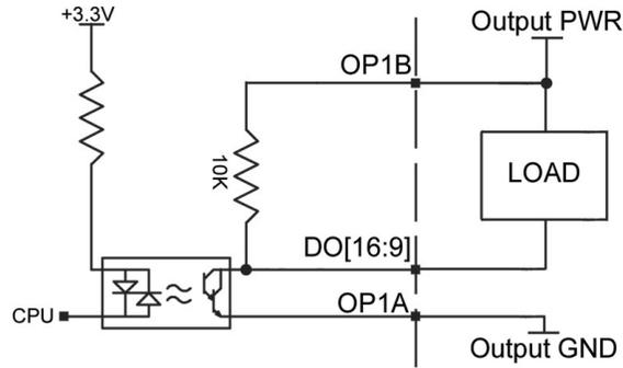
Figure 3.9: 25mA sinking wiring diagram for Bank 1, DO[16:9]
