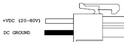
Figure 2.6: Power Connector used when controller is ordered without Galil Amplifiers
