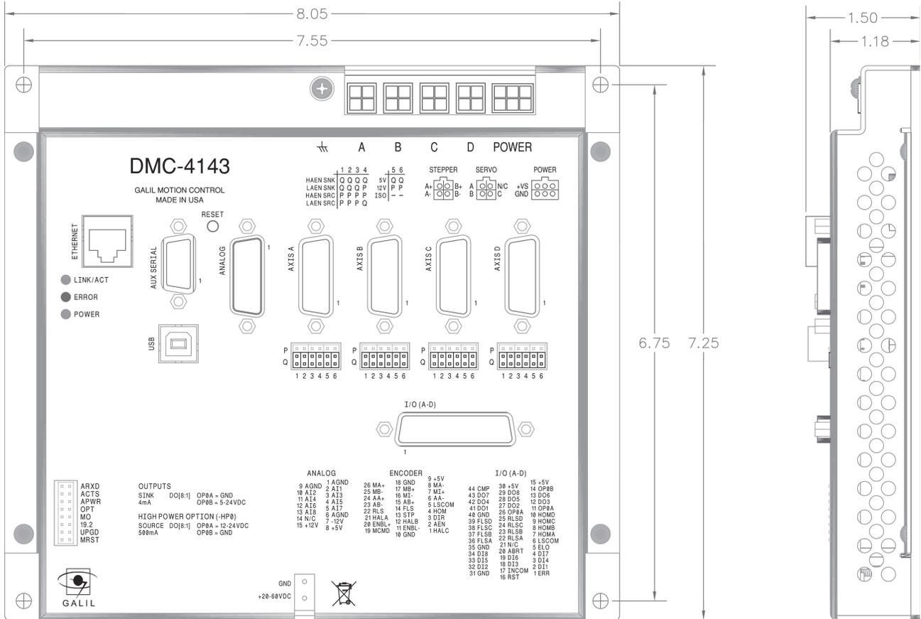
Figure 2.3: DMC-41x3-BOX4 Dimensions<sup>1</sup> (in inches) where x= 1, 2, 3, and 4-axis
