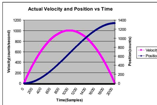
Figure 6.17: Actual Velocity and Position vs Time of Parabolic Velocity Profile
