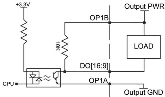
Figure 3.7: 4mA sinking wiring diagram for Bank 1, DO[16:9]
