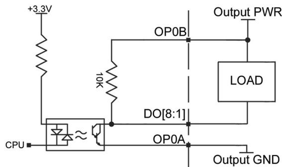
Figure 3.8: 25mA sinking wiring diagram for Bank 0, DO[8:1]
