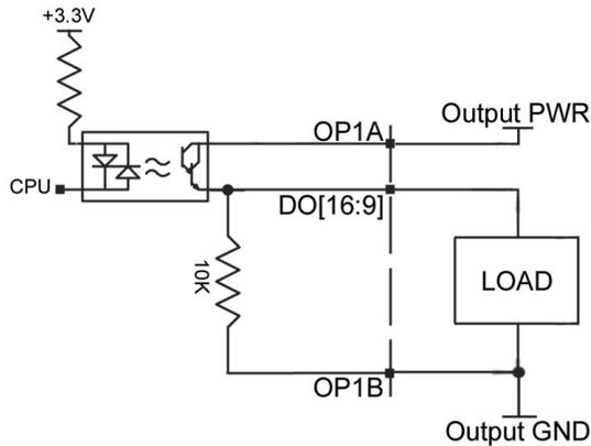
Figure 3.11: 25mA sourcing wiring diagram for Bank 1, DO[16:9]
