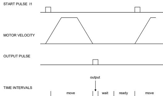
Figure 7.1: Motor Velocity and the Associated Input/Output signals
