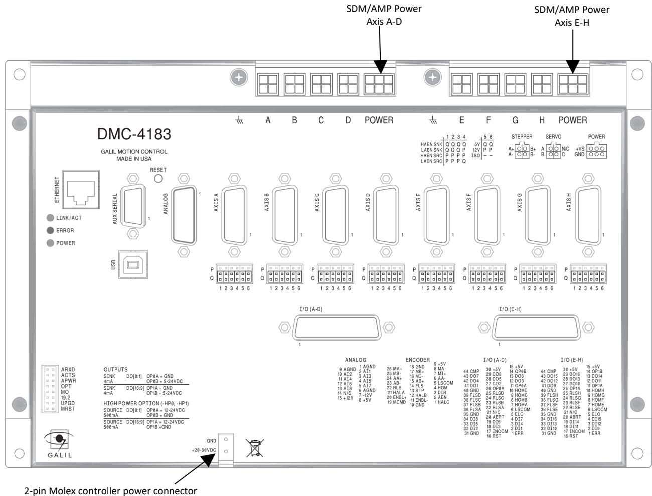
Figure 2.5: Power Connector locations for the DMC-41x3
