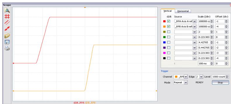
Figure 6.12: Velocity (counts/sec) vs. Time (msec) Ramped Gearing
