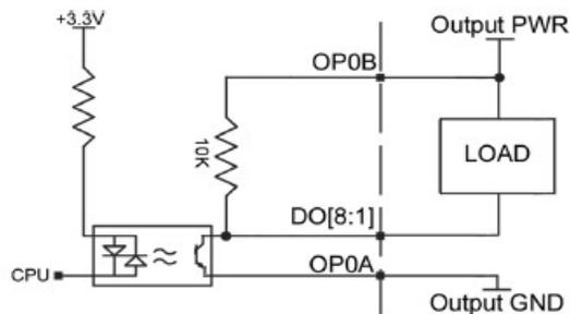
Figure 3.6: 4mA sinking wiring diagram for Bank 0, DO[8:1]
