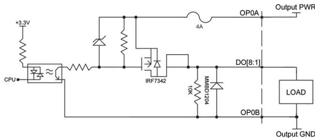
Figure 3.12: 500mA sourcing wiring diagrams for Bank 0, DO[8:1]
