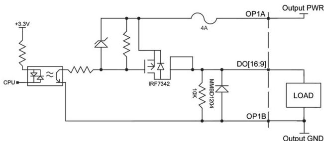
Figure 3.13: 500mA sourcing wiring diagram for Bank 1, DO[16:9]
