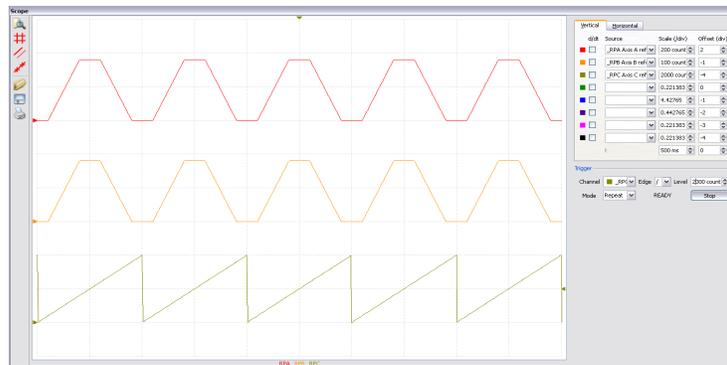
Figure 6.14: ECAM cycle with Z axis as master
