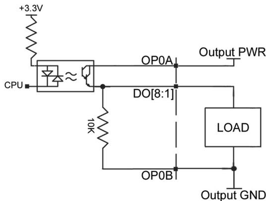
Figure 3.10: 25mA sourcing wiring diagram for Bank 0, DO[8:1]
