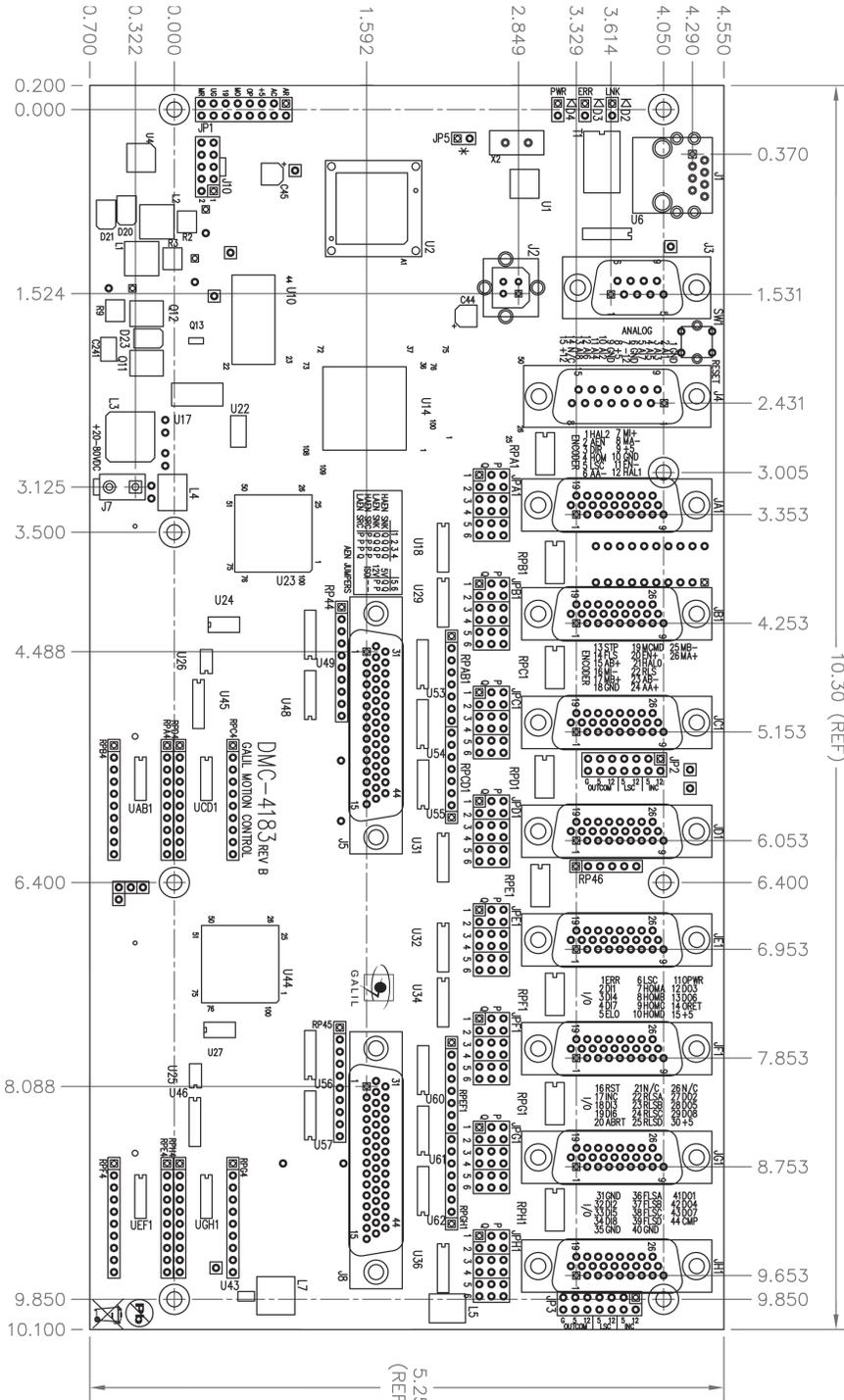
Figure 2.2: DMC-41x3 Dimensions<sup>1</sup> (in inches) where x= 5, 6, 7, and 8-axis
