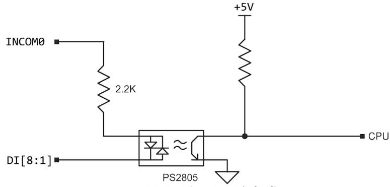
Figure 3.1: Digital Inputs 1-8 (DI[8:1])
