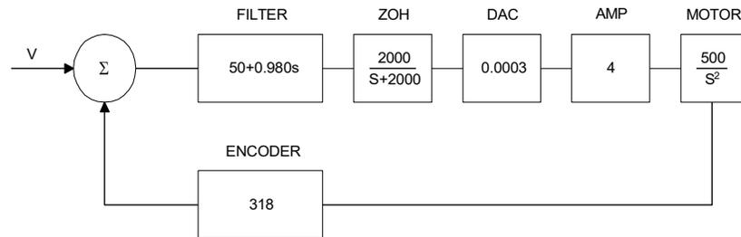
Figure 10.6: Mathematical model of the control system
